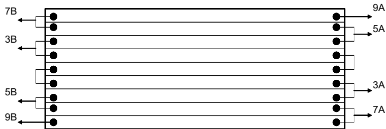
Fig. 3. Wiring of heating foils.
